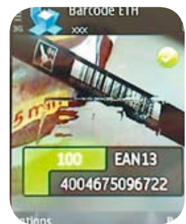
Scanning an EAN-13 bar code using the BATOO application developed by ETH Z, rich
